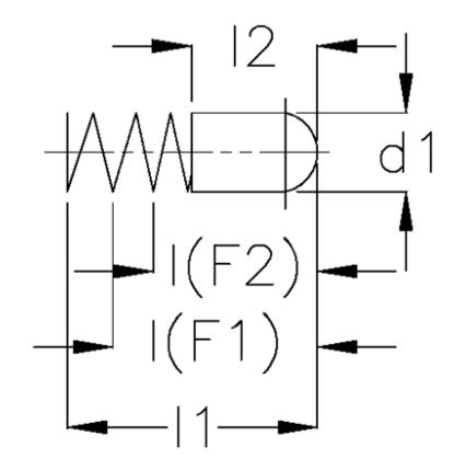
$\begin{array}{lll} d1 & = 3.0 \\ I(F1) & = 9.0 \\ I(F2) & = 8.7 \\ I1 & = 12 \\ I2 & = 6.0 \\ Spring pressure (F1) N = 6.2 \\ Spring pressure (F2) N = 6.8 \end{array}$
